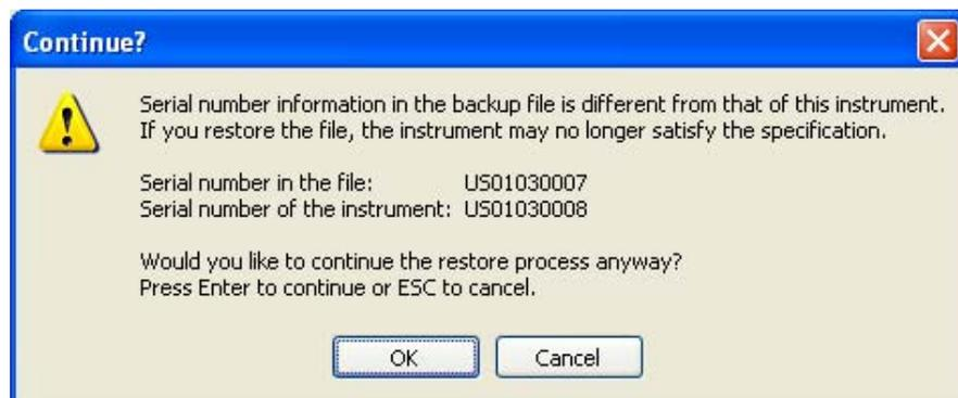
For the N9030A, the default restore location will be the internal F: drive which is a solid-state memory device located internally on the instrument. The default restore file will be the most recent file that matches the default backup file name format: AlignDataBackup\_N9030A\_<serial number>\_<date>.bak
